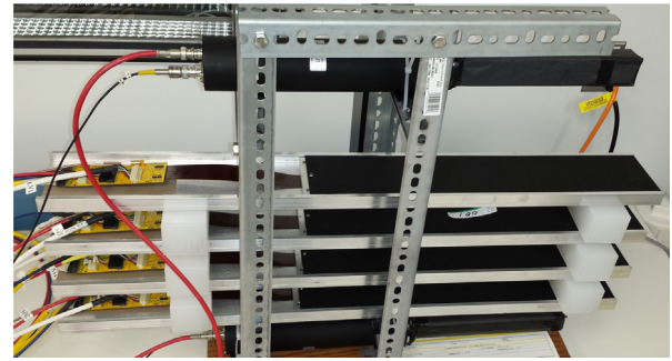
Fig. 85. The SVT cosmic test stand. Four SVT modules in their carrier boxes are mounted between the trigger paddles.
