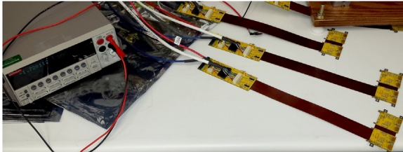
Fig. 19. Electrical test of the HFCBs.
