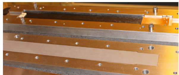
Fig. 23. Assembling the backing structure in the mold.
